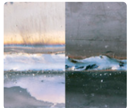
Descaled surfaces prior to welding lead to clean welding seams
